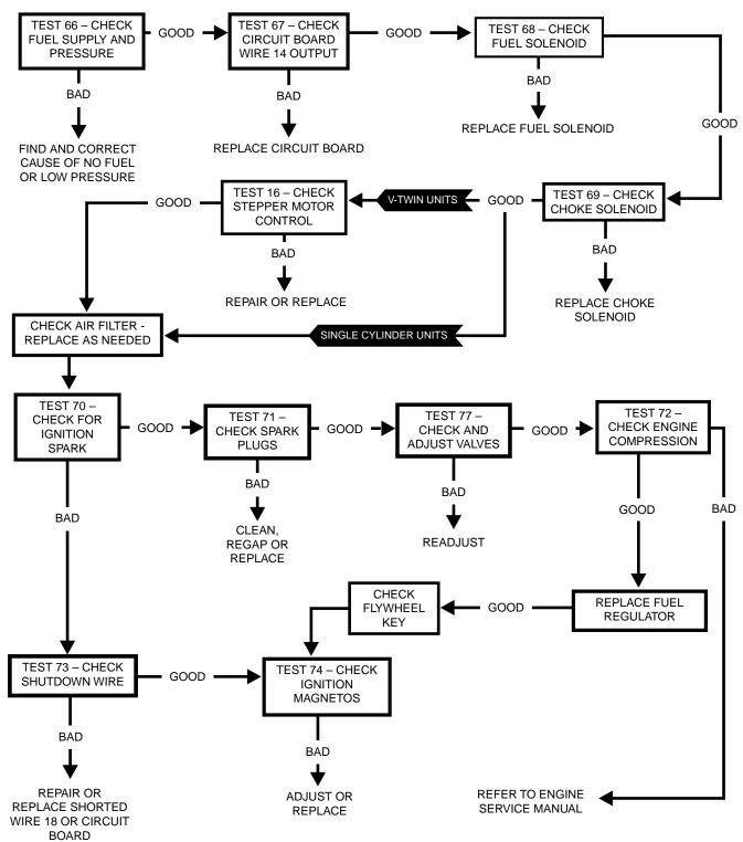
Problem 18 – Engine Starts Hard and Runs Rough / Lacks Power / Backfires
